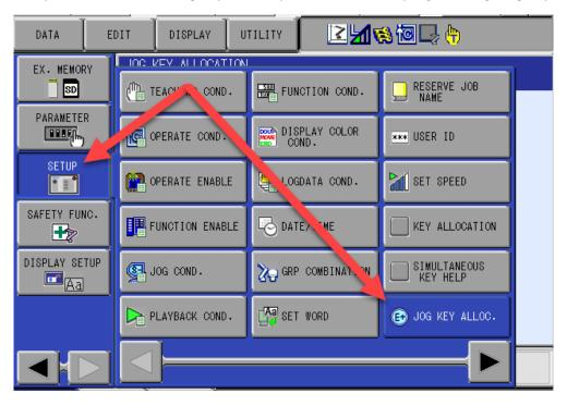
Once inside the Jog Key Allocation menu, setup of the extra axis can occur.
